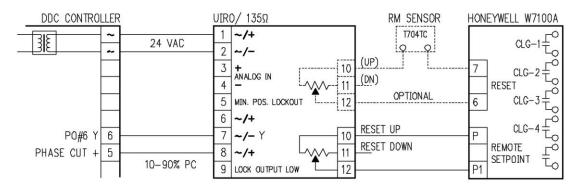
The UIRO can be field configured to accept STAEFA's phase cut signal and output a 3-wire resistance output that can be used in resetting a Honeywell W7100a series discharge temperature controller. This can be accomplished in two ways; first, provide a 0-135V up to 1000V resistance directly into the remote set point, the second directly resets the temperature input by adding resistance to the room sensor. A 135V resets controller by 13.5°F, 500V resets by 50°F, 1000V resets controller by 100°F.
