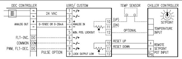
The UIRO can be used with an automation system to reset packaged chiller temperature controls equipped with remote input or remote set point potentiometers. The UIRO 3-wire output replaces the remote set point potentiometer and should be the same resistance value. Check the chiller specifications for reset resistance values for the desired °F of reset.
