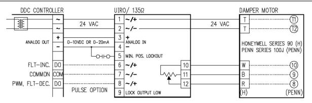
The UIRO can accept a variety of input signals and output a 3-wire resistance output that can be used to control a Honeywell or Penn actuator. A damper minimum position value can be added by using the auto/manual potentiometer. The minimum value can be measured between Tp3 and Gnd, (0 to 5VDC represents 0 to 100% of the output) and be disabled by connecting terminal 5 (minimum position lock out) to terminal 4 (common) allowing the actuator to close completely.
