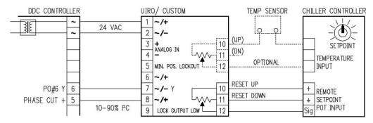
The UIRO can be used with an automation system to reset packaged chiller temperature controls equipped with remote input or remote set point potentiometers. The UIRO 3-wire output replaces the remote set point potentiometer and should be the same resistance value. For remote reset input check the chiller specifications for reset resistance values for the desired °F of reset.
